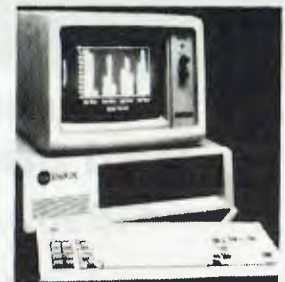
TAVA PC 256K Compatible PC 4/8 MHz. Switchable 2 x 320K slimline drives 1 x parallel, 1 x serial port, includes colour card.
